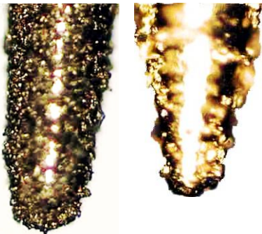
50um GPCD Probe Tip 10um GPCD Probe Tip (Zoom 481:1)
