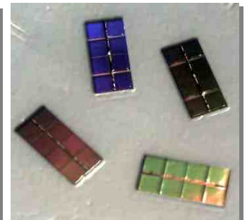
Extracted dice from original packaging ready to ship or ready for reassembly
