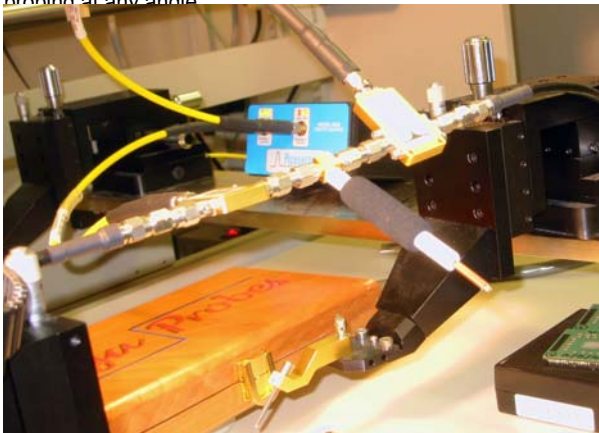
Fig. 5) Shows the DVT30-1MM GigaProbes™ directly hooked up the PSPL 4022TDT to generate a 30+ GHZ differential or single ended TDR pulse. This picture shows a differential TDR probing configuration. A micromanipulator can be used to hold the probe. The steel probe tips are very rugged and resist damage.
